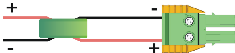
Fig. 6. Mounting the ferrite cores on the DC cables to the amplifiers
