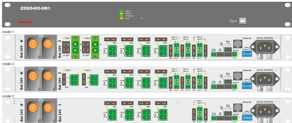
Fig. 2. View of ZDSO400-DR1 front panel and three variants of rear panel.
